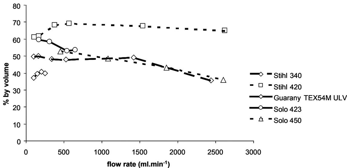
Fig 2. Droplet size spectra of mistblowers used on cocoa: % of spray volume in the range 55-126 µm.
