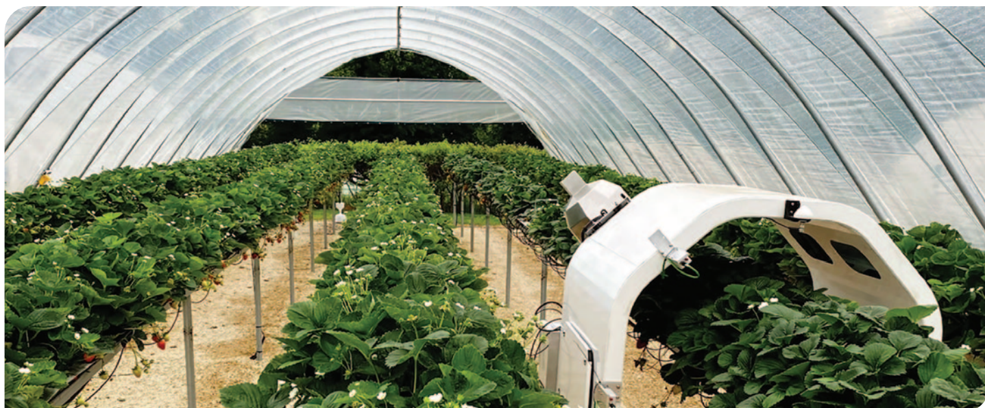
A Thorvald robot treating a strawberry crop with UVC light to control powdery mildew.
